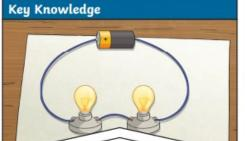
only flow around a complete circuit that has no gaps. There must be wires connected to both the positive and negative end of the power supply/battery.
